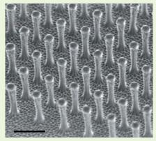
A scanning electron micrograph of microfabricated polyimide hairs like those employed on gecko tape. Scale bar is 2 µm.
