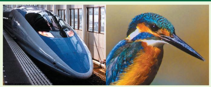
The design features of Japan's Shinkansen 500-Series exemplifies biomimicry in action. Its overhead pantograph sports serrations were modeled on the design of owl plumage to reduce air resistance noise, and the air piercing nose cone design was inspired by the kingfisher's beak. From the Swiss-Japan Assoc. for Engineers and Scientists
