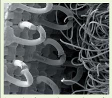
A scanning electron microscope image of Velcro's hooks and loops (370 micron view).
